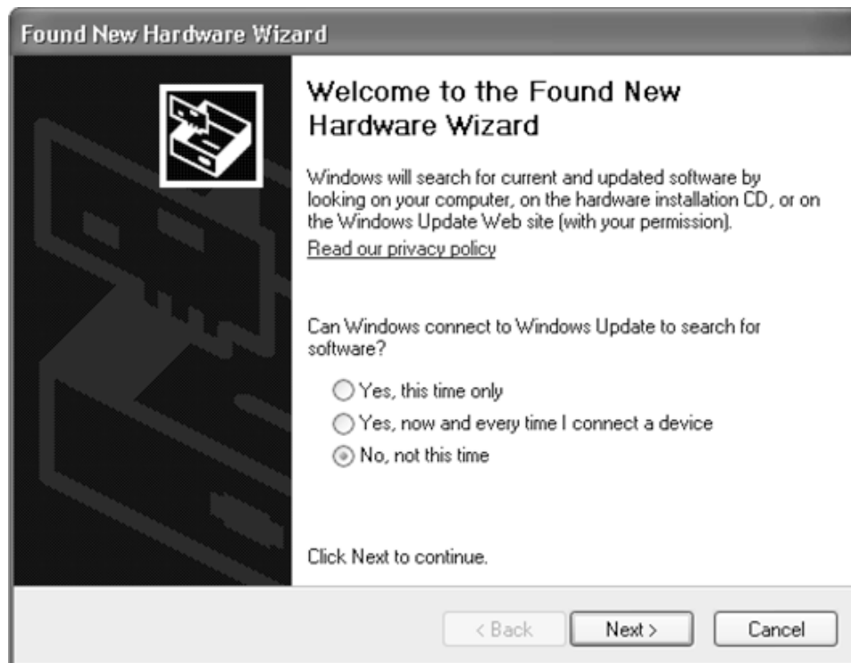
Figure 8. Found New Hardware Wizard—Start Hardware Driver Installation (select No, not this time , and click Next to continue)
